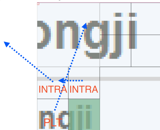
Figure 2 Decoder-Side Block/Motion Vector Derivation (green block indicating current CU to be encoded. Neighboring Intra or PLT block can provide additional block vector or motion vector)
